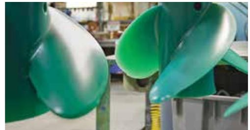
Mercury produces the best performing propellers. All stainless steel props begin as a perfect wax replica of the final product.
