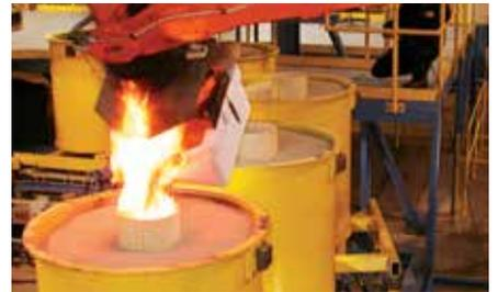
Mercury's exclusive pressurized lost-foam foundry produces more-intricate castings that require fewer fasteners for lighter weight and increased reliability.
