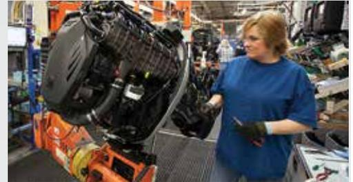
Ergonomic assembly fixtures allow Verado technicians to focus on the details, engine after engine, all shift long.
