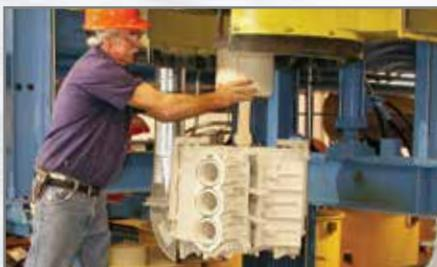
Mercury's exclusive pressurized lost-foam foundry produces components that are stronger, lighter and require fewer fasteners for top-notch reliability, strength, and lower weight.
